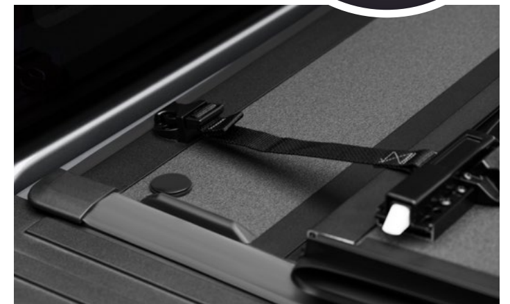
BUCKLE SYSTEM SECURES COVER IN FOLDED POSITION
