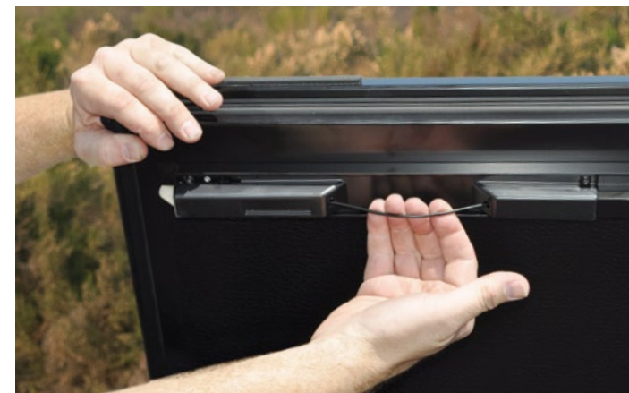
ACCESS RELEASE CABLES ON EITHER SIDE
