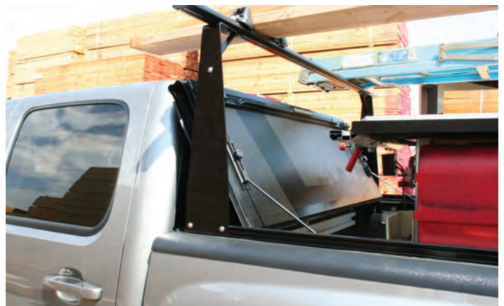
COVER FLIPS UP TO HAUL LARGE EQUIPMENT
