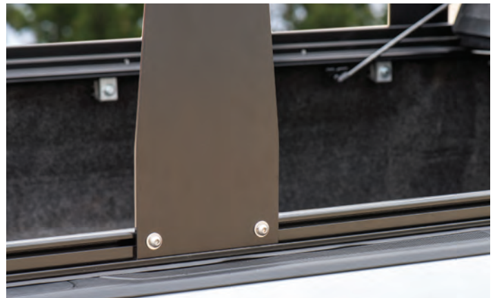
RACK UPRIGHTS EASILY SLIDE ALONG CARGO RAILS
