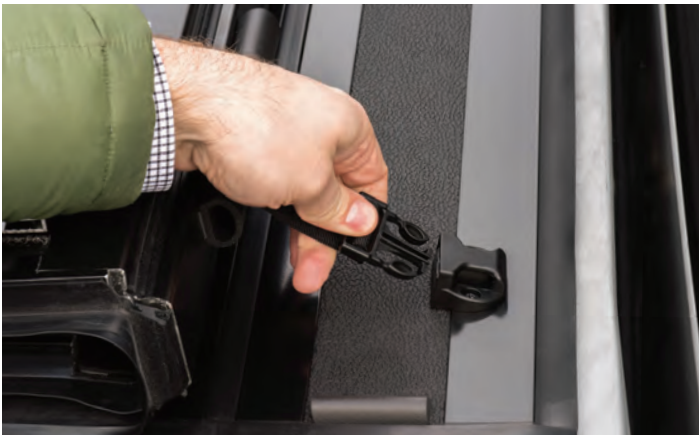
BUCKLES SECURE COVER IN FOLDED POSITION
