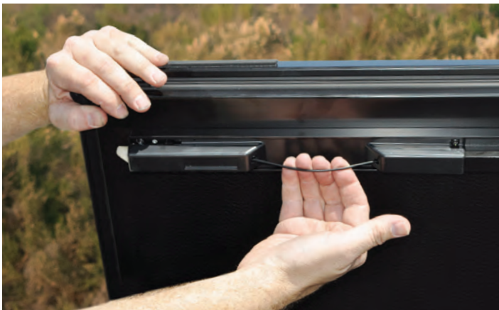
ACCESS RELEASE CABLES ON EITHER SIDE
