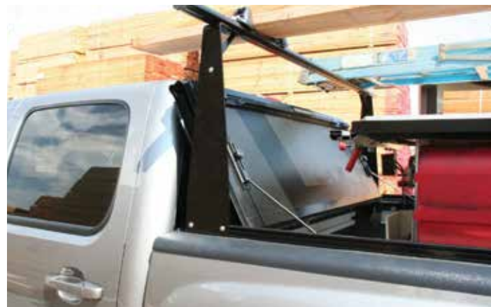
COVER FLIPS UP TO HAUL LARGE EQUIPMENT
