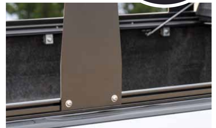
RACK UPRIGHTS EASILY SLIDE ALONG CARGO RAILS
