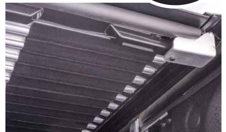
UNDERSIDE REVEALS STRONG ALUMINUM SLATS
