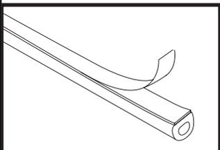
Roll the cover open and place the D shaped bumpers to the aluminum underside where they will prevent contact if the cover is rolled all the way open. The straps will hold the cover off the cab and glass when secured.
