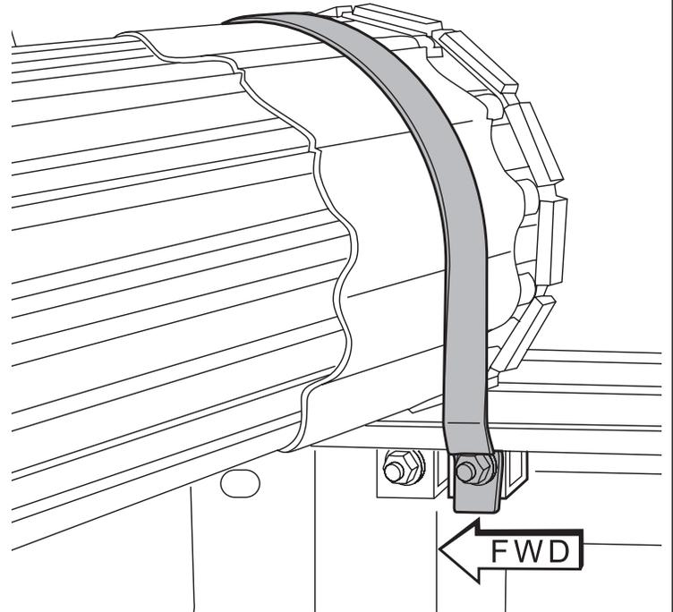
Mount the strap clamp assembly as far forward on the rail as possible and tighten. Repeat on opposite side.
